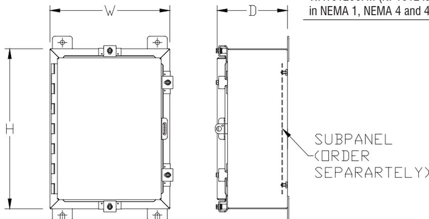
Note: Do NOT use NPxxxxC subpanels in NEMA 1, NEMA 4 and 4X, and NEMA 12 enclosures. For example: Subpanel NP1612C will not fit enclosure. WA161206FM (NP1612 is the correct subpanel). Only use NPxxxx subpanels in NEMA 1, NEMA 4 and 4X, and NEMA 12 enclosures.
