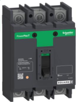
**Circuit breaker, PowerPact Q, 125A, 3 pole, 240VAC, 10kA, lugs, thermal magnetic, 80%**
