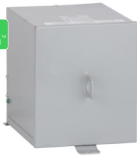
Transformer, dry type, encapsulated, 5kVA, 1 phase, 240x480V primary, 120/240V secondary, 13B, 115C rise
