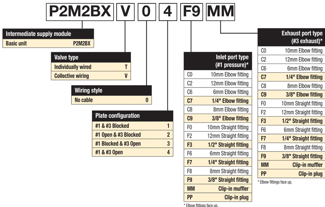
**Moduflex Add-A-Fold Assembly Model Number Index**
