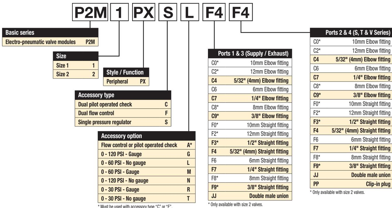
**Intermediate Supply Module Model Number Index**
