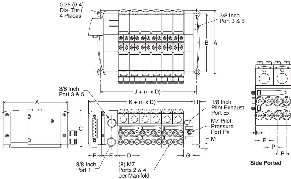
**25-pin, D-Sub with Isys Micro Valves, Bottom Ported**
