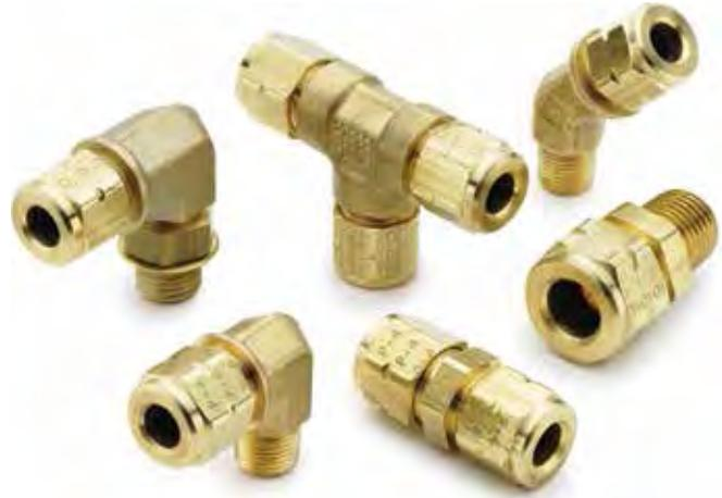
Parker's Vibra-Lok Fittings provide a positive reliable seal under vibration conditions, mechanical shock or tube movement. The sleeve cushions the tubing, permitting the tubing to flex back and forth in the fitting. The seal design compensates for tube misalignment and tube surface defects.
