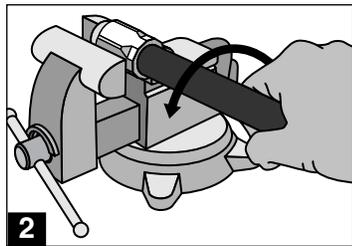
2. Place socket in vice and screw in hose counter-clockwise until hose bottoms. Back hose out 1/2 turn.
