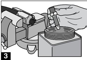
3. Dip hose end of nipple into Hoze-Oil or other heavy oil up to the hex. When assembling fittings of 316 stainless steel lubricate the threads of both the socket and nipple with Dow Corning Molykote G-n or equivalent metal assembly lubricant.
