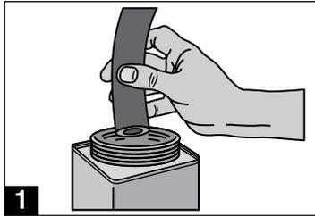
1. Identify over all length (OAL) of hose assembly and the cut off allowance (COA) length of fitting(s) on hose ends by use of the fitting data table. Properly measure, mark and cut hose to desired length using fine tooth hacksaw or a cutoff machine. Dip hose end into Hoze-Oil (See Section C) or heavy oil.
