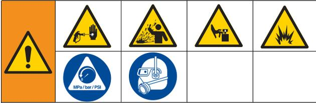
This equipment stays pressurized until pressure is manually relieved. To help prevent serious injury from pressurized fluid, such as skin injection, splashing fluid and moving parts, follow the Pressure Relief Procedure when you stop spraying and before cleaning, checking, or servicing the equipment.
