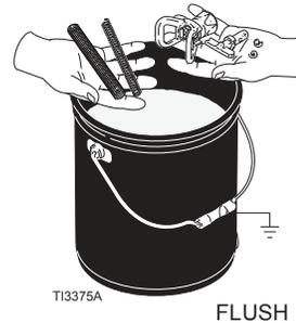
5. Place siphon tube set in grounded metal pail partially filled with flushing fluid. Attach ground wire to true earth ground. Perform Startup steps 10 - 17 (see page 13) to flush out paint in sprayer. Use water to flush water-base paint and mineral spirits solvent (also called white spirit) to flush oil-base paint.
