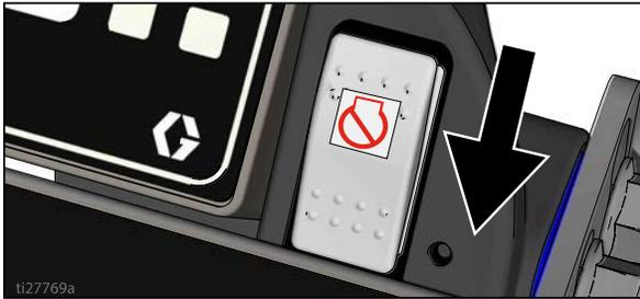
15. Increase pressure control enough to start pump. Allow fluid to circulate for 15 seconds.
