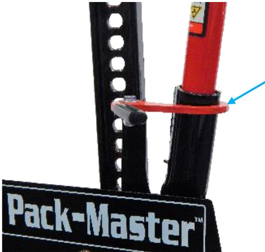
4. Disengage the handle lock hook, and then pump the jack handle up and down to lower the ram plate for compaction.
