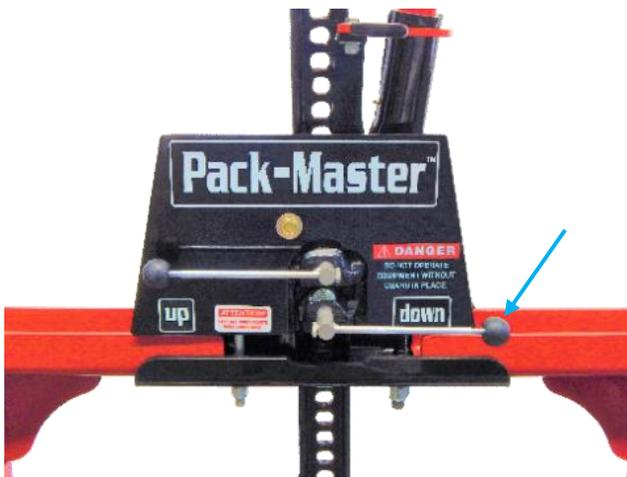
3. Then rotate the upper lever to the **down** position.
