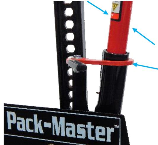
2. To begin compacting waste, rotate the lower lever to the **down** position.
