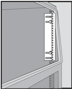
Symmetrical Rack Angles have through-holes in mounting surfaces for mounting rack equipment. Rack Angles with through-holes accommodate either English or metric cage nuts.
