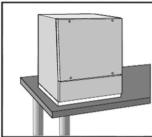
Base closes off open bottom of ProLine Sloped-Front HMI Enclosures that are table-top mounted or suspended from overhead. Base includes a ground stud. Foam-in-place gasket assures a water-tight and dust-tight seal. A top support bracket can be installed inside a 600-mm wide base for reinforcement when a Compact Series 4 System 80 is attached from below.
