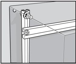
Mounting Channels provide mounting framework for installing DIN rails and grid straps at various positions within the enclosure. Channels can be mounted vertically or horizontally to collar studs or to the slide mechanisms of the adjustable-depth mounting kit.
