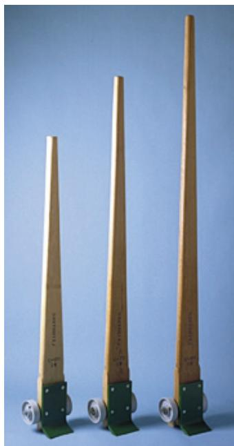
Fairbanks' C Series lever dollies feature kiln-dried, 1-3/4" thick, oak handles with rounded edges. Reversed beveled nose iron is 6" wide x 3" deep and bolted to the handle and heavy-duty axle. Handle lengths are 60", 72" and 84". Wheel options are: Semi-steel with plain bore (IW), solid hard rubber with Delrin bearings (HRI), polyurethane mold-on cast on and rubber mold-on cast iron (RT). Lever dollies typically used in pairs.
