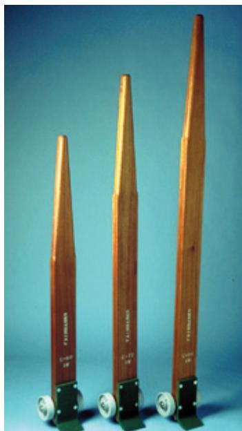
These husky, durable E Series lever dollies easily get under extremely heavy loads with the reversed beveled nose iron, which is bolted to the handle for greater strength. E Series lever dollies have a 5" wide x 3" deep nose iron and the oak hardwood handles have smooth, rounded edges. Wheel options are: Semi-steel with plain bore (IW), polyurethane mold-on cast iron (PO), and rubber mold-on cast iron (RT). Lever dollies typically used in pairs.
