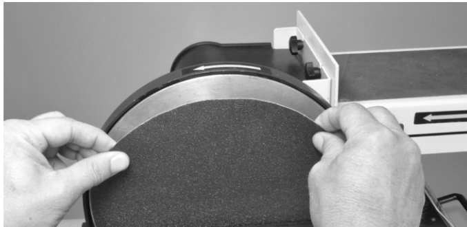
Figure 6 - Mount sandpaper disc.
