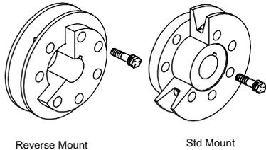
7. Position the bushing - product assembly axially on the shaft such that it is aligned with its running mate. Be sure to check for adequate clearance between the assembly and other nearby components if applicable. If the bushing has a setscrew over the keyway, tighten it to the torque value in Table 2.
