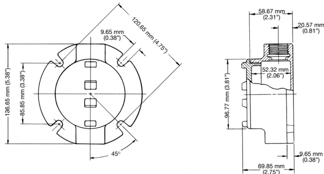
♦ In Class I, Division 1, Group B atmospheres, all conduit runs must have a sealing fitting (not supplied) field-installed adjacent to the enclosure.
