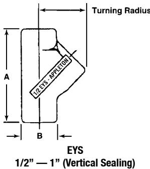
\* Per NEC 501.15(C)(6), seals in Class I, Division 1 and 2 must be limited to conductor fill of 25% of cross sectional area of a rigid metal conduit of the same trade size unless approved for higher percentage fill. See 40% fill sealing fittings.
