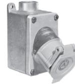
**Factory sealed receptacle/switch interior.** Switch is an integral part of receptacle interior, contained in an aluminum sleeve. Protective xylan coating on inside of sleeve provides smooth "rotating" action of internal switch, which is activated by rotating plug in receptacle. Entire aluminum sleeve is sealed at both ends with neoprene O-rings to protect receptacle/switch interior against moisture.
