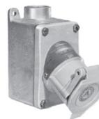
**Factory sealed receptacle/switch interior.** Switch is an integral part of receptacle interior, contained in an aluminum sleeve. Protective xylan coating on inside of sleeve provides smooth "rotating" action of internal switch, which is activated by rotating plug in receptacle. Entire aluminum sleeve is sealed at both ends with neoprene O-rings to protect receptacle/switch interior against moisture.
