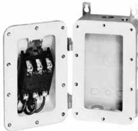
Solderless lugs are provided for line connections, and receptacle is prewired to the load side of breaker. Cover-mounted components leave entire enclosure space free for pulling of line conductors and wiring.
