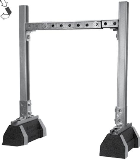
The HBS-DSAW Series is designed specifically for supporting duct work. The telescopic cross beam provides easy size adjustments. A wide range of support widths are provided from 19<sup>1</sup>/<sub>4</sub>" to 103<sup>5</sup>/<sub>8</sub>"
