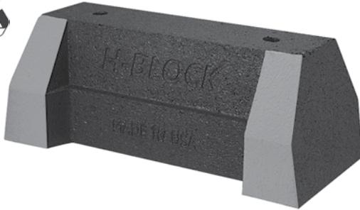
The HBS-Base Series is UV resistant and suitable for installation on most types of roofing material or other flat surfaces. Can be used as a curb (sleeper) replacement. Screw fasteners can be used to attach one or two hole pipe straps or a piece of strut (not included).
