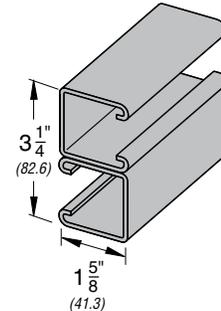
Our welded channels are spot welded 2" (50.8mm) on center, dimensions shown are for welded variations of any channel with or without slotted holes.
