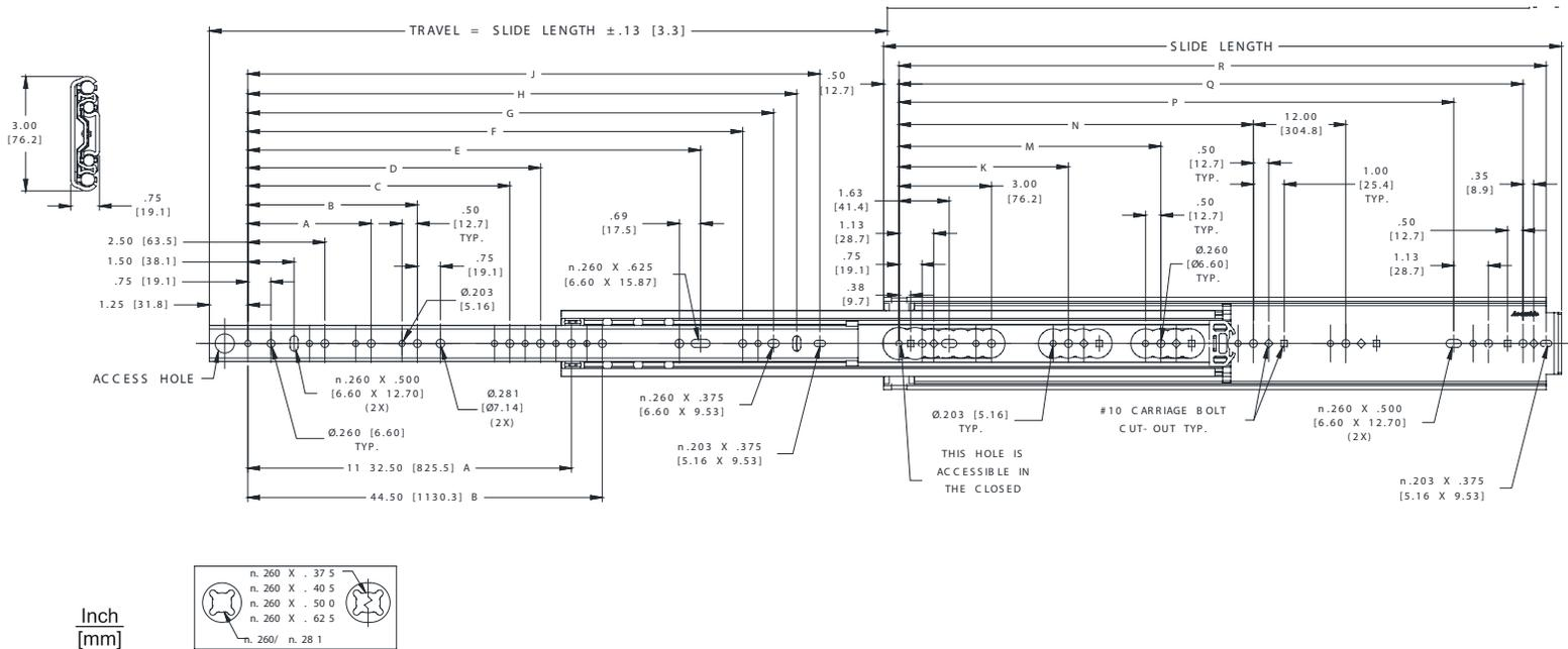
Note: Maximum screw head of .190" [4.8mm] high by .500" [12.7mm] diameter necessary to clear traversing members.
